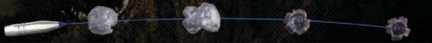
Bullet upsets captured from 200-grain 300 Win. Magnum load, P300WTA1
